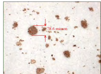
Sample measurement (in this case, the measurement considers a single specific particle)
